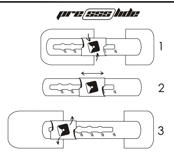
PRESS-SLIDE SYSTEM allows to adjust the required brace length in this case:
